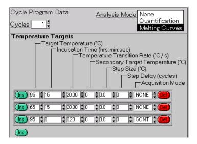
(4) The cycling parameters should be set according to the following window. Analysis and Acquisition mode of the cooling step must be set at "Non".
