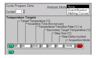
(2) The cycling parameters should be set according to the following window. Analysis mode of the PCR step must be set at "Quantification". And Acquisition modes of 95°C and 60°C must be set at "None" and "Single", respectively.
