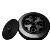
NO. 6 8x100ml Fixed-angle Rotor Max Speed : 12000rpm Max RCF : 19830xg Tube size : Φ37x123mm
