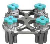
NO. 3-1 16x15ml Swing-out Rotor Max Speed : 5000rpm Max RCF : 4620xg Tube size : Φ17x121mm
