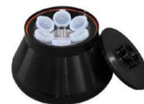
NO. 4 6x100ml Fixed-angle Rotor Max Speed : 14000rpm Max RCF : 23600xg Tube size : Φ37x123mm
