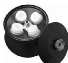
NO. 7 4x300ml Fixed-angle Rotor Max Speed : 14000rpm Max RCF : 28150xg Bottle size : Φ61x136mm
