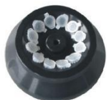
NO. 1 12x1.5ml/2.2ml Fixed-angle Rotor Max Speed : 16000rpm Max RCF : 17800xg Tube size : Φ11x42mm
