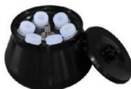
NO. 6 6x300ml Fixed-angle Rotor Max Speed : 10000rpm Max RCF : 16750xg Bottle size : Φ61x136mm
