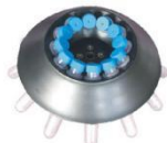
12x20ml Fixed-angle Rotor
