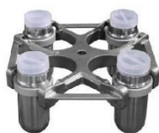
NO. 2 4x100ml Fixed-angle Rotor
