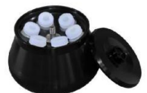
NO. 4 6x300ml Fixed-angle Rotor Max Speed : 12000rpm Max RCF : 24110Xg Bottle size : Φ61x136mm
