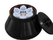
NO. 5 6x100ml Swing-out Rotor Max Speed : 16000rpm Max RCF : 30910xg Tube size : Φ37x123mm
