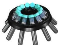
NO. 1-1 12x15ml Fixed-angle Rotor Max Speed : 5000rpm Max RCF : 3550xg Tube size : Φ17x121mm
