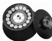
NO. 3 16x10ml Fixed-angle Rotor Max Speed : 16000rpm Max RCF : 27500xg Tube size : Φ16x86mm
