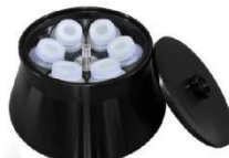
NO. 3 6×500ml Fixed-angle Rotor Max Speed : 8000r/min Max RCF : 11880xg Bottle size : Φ74×170mm
