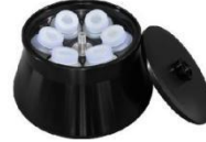
NO. 9 6x500ml Fixed-angle Rotor Max Speed : 10000rpm Max RCF : 18590xg Bottle size : Φ74x170mm
