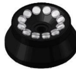
NO. 7 12x50ml Fixed-angle Rotor Max Speed : 14000rpm Max RCF : 30070Xg Bottle size : Φ29x119mm
