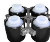
NO. 8 4x750ml Swing-out Rotor Max Speed : 4000rpm Max RCF : 3500xg Bottle size : Φ100x141mm
